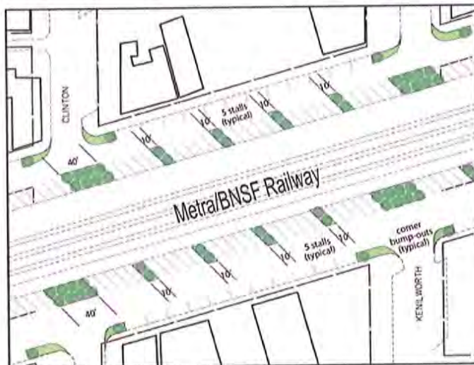
Proposed Typical Block Plan Outside of the Immediate Harlem Avenue, Berwyn ("Depot District"), and LaVergne Station Areas
