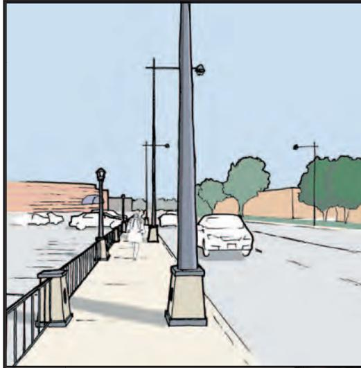
Sketch shows concept for a decorative railing system which is used to enclose large parking lots and define a street edge along the sidewalk. Decorative street lamps are combined with the post for the railing. Existing condition at right.
