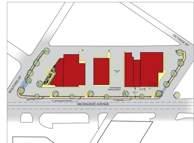
Figure 3. An illustrative plan for improving sites configured with a single bay of parking. Access is controlled and a consistent sidewalk provided.
