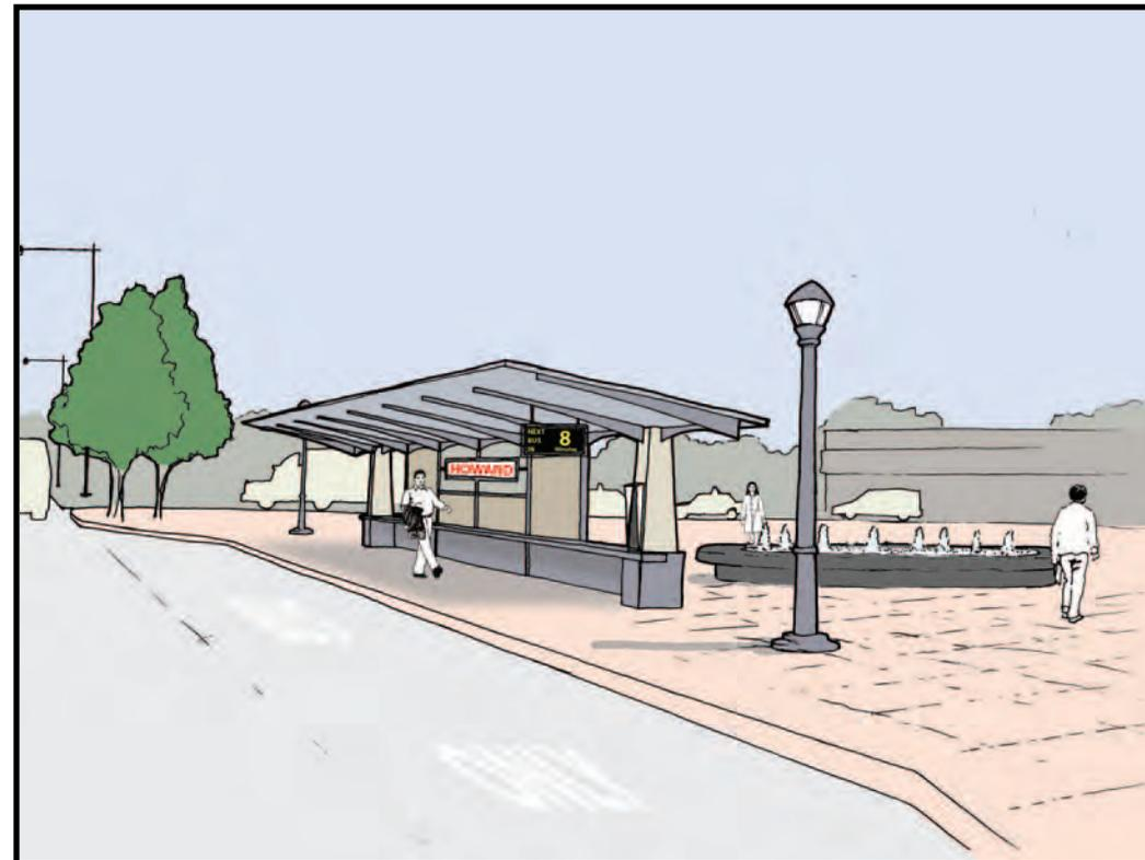
Figure 30. Illustrative sketch of a BRT station on the triangle between Howard and Harlem shows the dedicated bus-only lane along Milwaukee Ave. The BRT station includes a large canopy and platform (or boarding area) and a display showing real-time information on when the next bus will arrive (reading 8 minutes).
