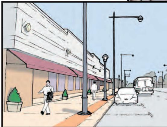
Sketch shows how a consistent sidewalk and new lane for parallel parking can be installed in existing space between building facades and the drive lane. Existing condition at right.
