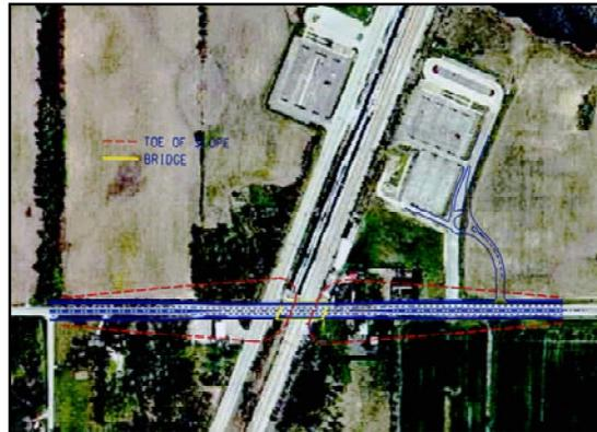
FIGURE 26: CONCEPTUAL DIAGRAM OF THE PROPOSED UNIVERSITY PARKWAY OVERPASS
