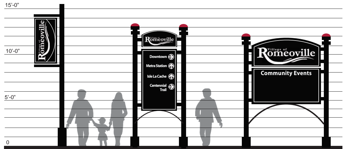
THE SIGNAGE FAMILY PROVIDED IN SECTION 3 INCLUDES BANNERS (LEFT), WAY-FINDING SIGNS (CENTER), AND GATEWAY/EVENTS SIGNS (RIGHT)
