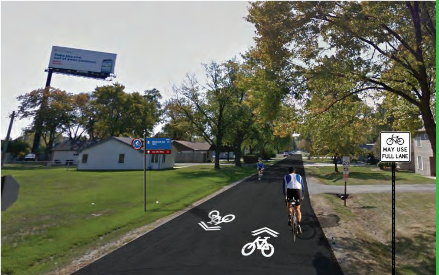
Shared Use route visualization at Ridgeland and Nagle Avenue including sharrow markings and signage
