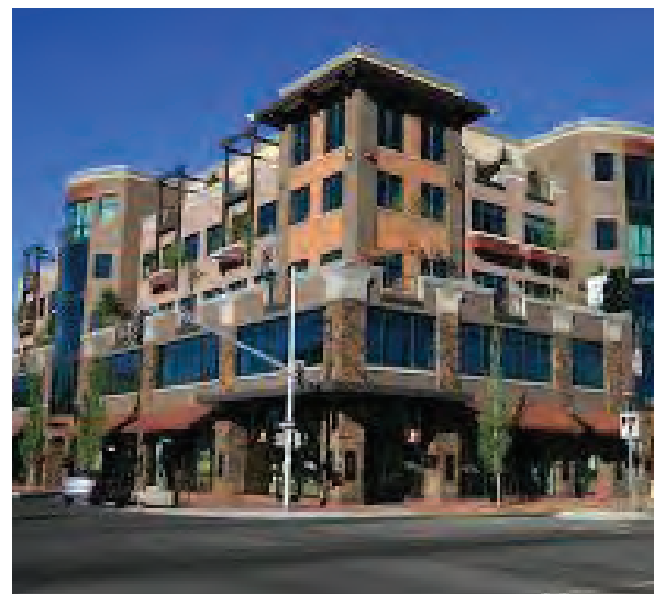
Upper floor units are set back behind ground floor spaces providing articulation and interest in the building facade.
