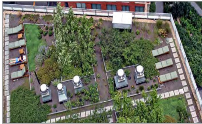
Two examples of green opportunities to explore in the proposed Town Center: (1) Permeable pavers can help stormwater infiltrate through the pavement and into the soil below (left); and (2) A green roof can help a building reduce energy consumption, reduce the urban heat island effect, and provide a rooftop outdoor space (right).
