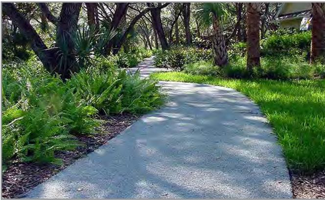
Although still a hard surface, pervious concrete allows water to flow through the material more freely, meeting EPA stormwater management standards.
