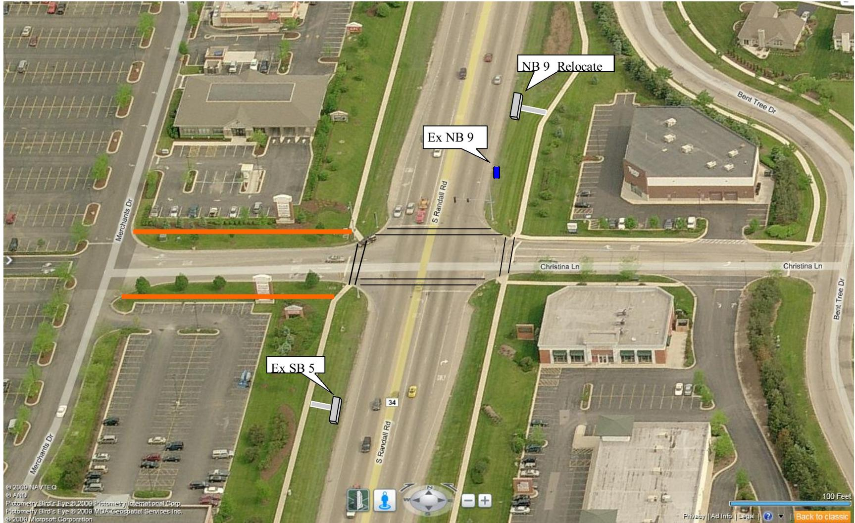
**Tier 1:** Relocate existing NB 9 stop, add bus shelter, add crosswalks and add walkway to connect to existing sidewalk. Add Bus shelter to existing SB 5 stop.
