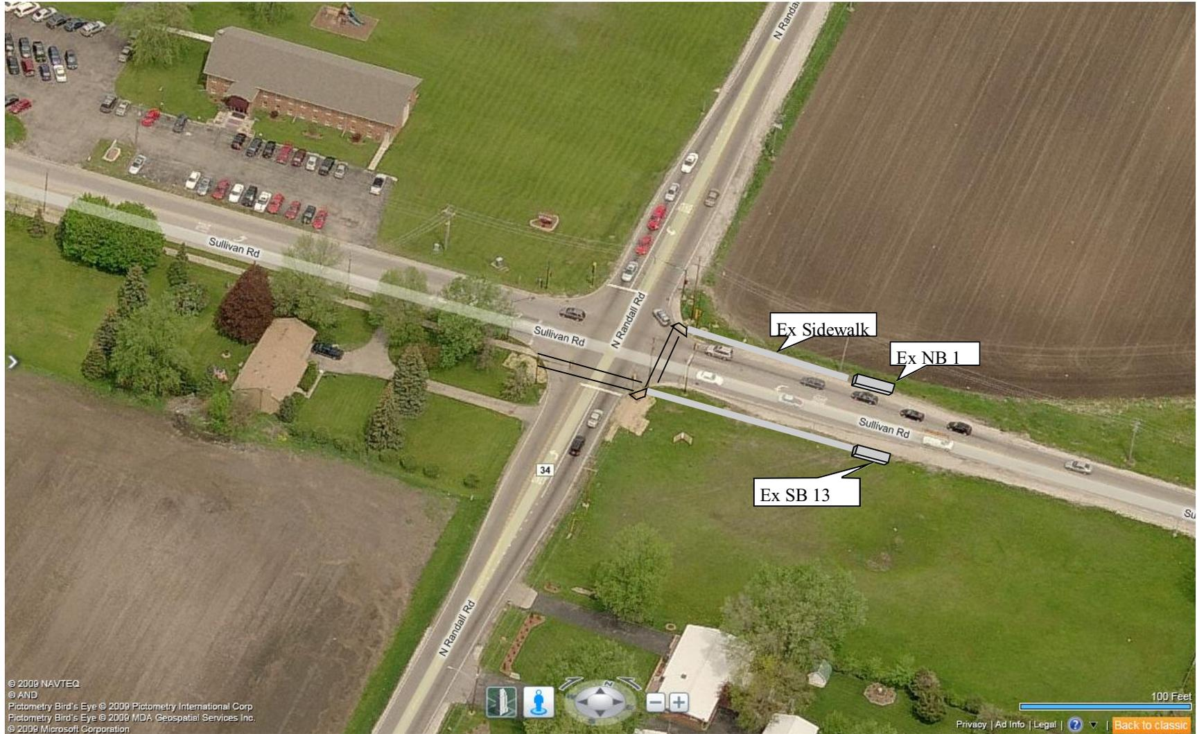
**Tier 1:** Maintain location of existing NB and SB stops, add bus shelters, add sidewalks, crosswalks, and access ramps.
