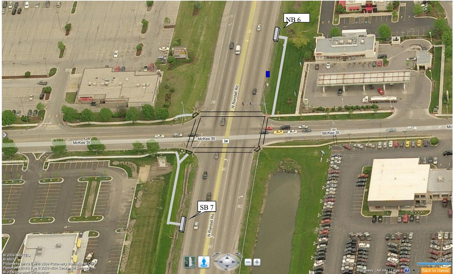
**Tier 1—Build bus shelters and relocate exist stops to meet Pace Stop Location Guidelines, add crosswalks, construct walkway to connect to existing sidewalks.. AT SB 7, there exists a big slope and ditch, culvert may be extended or build sidewalk to bridge over ditch area**
