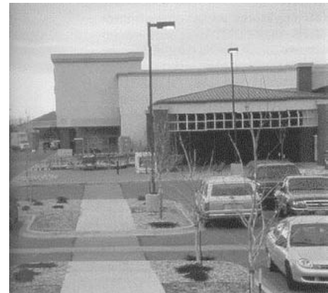
Parking areas should incorporate distinguished, identifiable pedestrian walkways to create a more pleasant and safer pedestrian experience.
