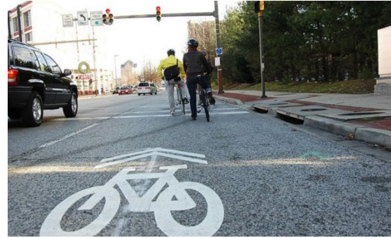
Example of Class III “Bike Sharrow” (City of Oakland, CA). Source: CityLab, 2015; online.
