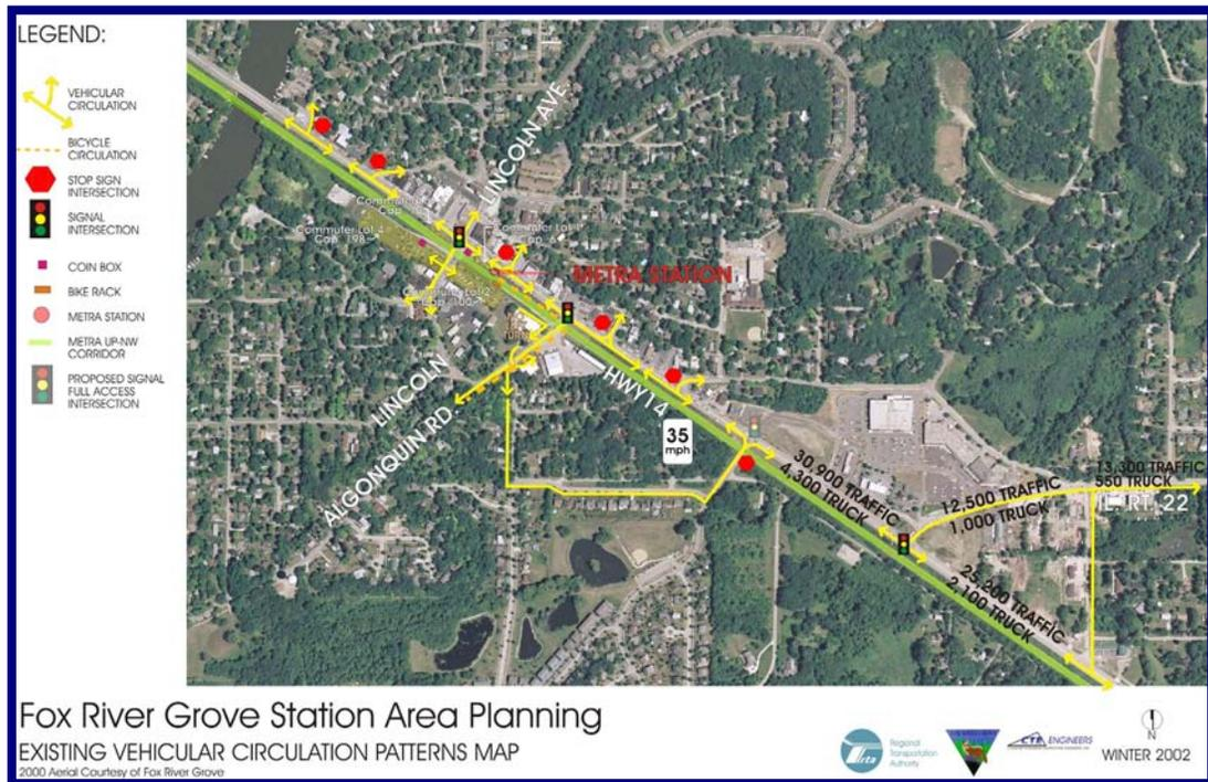
Figure 5 illustrates the existing vehicular circulation patterns in the Fox River Grove Metra Station area. The average daily traffic and truck traffic numbers are also shown in the figure. More information on the existing traffic in the area is available in Chapter 4: Transportation & Transit.
