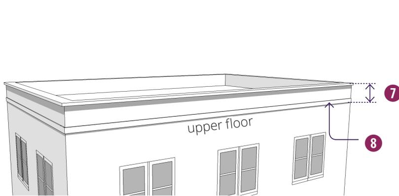
Figure 9-4D-20. Parapet Cap
