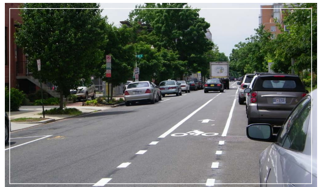
Provide clear bicycle markings to encourage cycling
