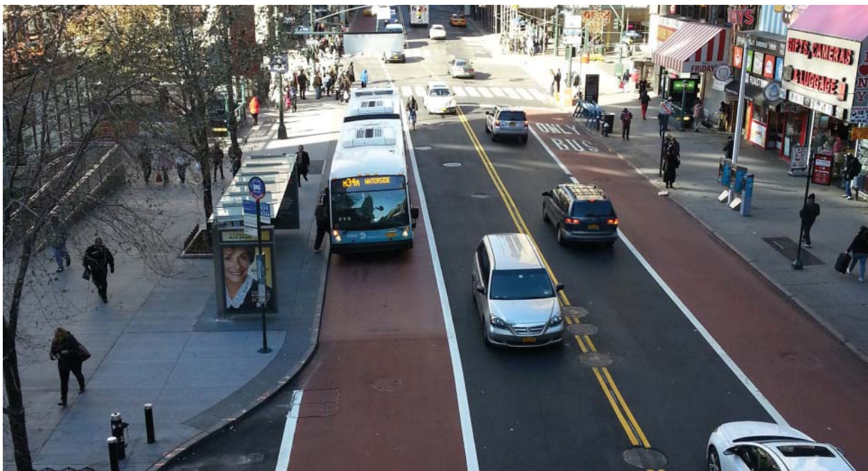
Figure 21: Example of a Dedicated Bus Lanes
